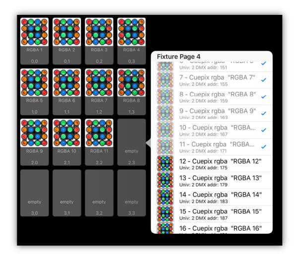
In the example above a 4 X 4 matrix has been created using individual RGBA LEDs from an Elation Cuepix blinder. In this example the fixture was patched as 16 separate RGBA LEDs rather than one large 64 channel fixture simply for convenience. If it had been patched as one large fixture you would only need to assign it to the first box and the rest of the pixels would have been filled in automatically. Each box shows the fixture's button name and image as well as the row and column number.
